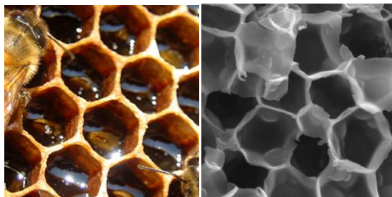
Fig 3 Nanoscale polymeric structures have been created spontaneously which show a remarkable parallel with the honeycomb structures created by bees whose constructions are about a million times larger.
